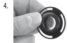
Remove the clutch disc (8) & spacer (9) out of the hub. Look at the two sides of the disc.
