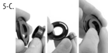
Pop out the Clutch Disc Spacer, Flip clutch disc to Cassette Mode (ramps face toward the hub), insert Disc Spacer back into the clutch disc with flanged end facing the driver & insert back into hub w/ clutch disc spacer, making sure the spring & all components are in the correct position.
