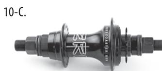
Thread the cone nut back onto the hub. Tighten with the 8mm allen inserted into the non drive side of the axle & the 21mm spanner wrench on the cone nut. Spin the hub & makes sure everything is moving freely & there is no rubbing or interference. Reinstall the wheel & you are on your way.
