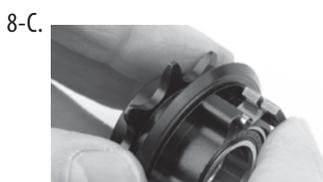
After the pawl & spring is out of the driver, insert the expansion spring in the same place that the previous spring came from. Be sure to insert the spring with the long side facing the pawl side. After the spring is loaded depress the spring with your finger & slowly reinsert the pawl. Now repeat for the other pawls.
