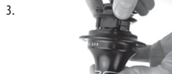
To prevent losing any parts, hold the hub so that the drive side is facing up. Slowly wiggle & pull the driver (13) off of the axle.
