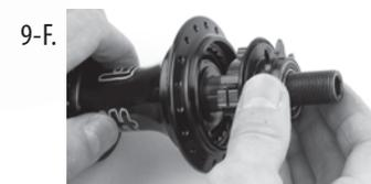
Slowly take the driver & slip it over the axle & slide it all the way back into the hub. Slowly turn the driver as you put it into the hub body to make sure the clutches are aligned in their correct position.
