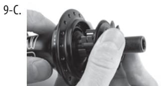
Carefully, take the reassembled driver & slip it over the axle & slide it all the way back into the hub. You might have to wiggle & turn the driver into position because of the tight tolerances.
