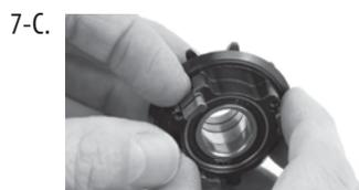
Remove the spring by slipping your fingernail under the pawl & lift the spring so that you can hold it with your finger. Now slowly pull the pawl out of the driver. Then, slowly pull the retention spring out of the driver.
