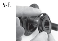
Pop out the Clutch Disc Spacer, Flip clutch disc to Freecoaster Mode (ramps face toward the driver), insert Disc Spacer back into the clutch disc with flanged end facing the driver & insert back into hub w/ clutch disc spacer, making sure the spring & all components are in the correct position.
