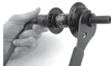
Insert 8mm allen wrench into non drive side of axle. On the drive side, loosen the 21mm cone nut (16) beside the driver & completely remove the cone nut from the axle.
