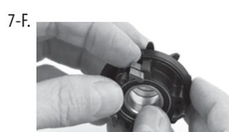
With the driver facing you depress the expansion springs with your finger & remove the pawls.
